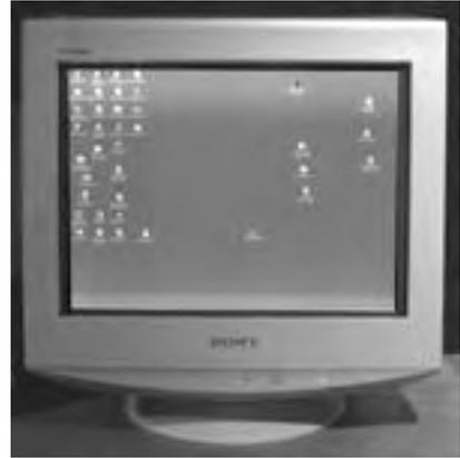
Currently CRT displays (See the example shown at the left.) are less expensive, especially for larger screen sizes. And, the overall image quality may be a bit better and colors more accurate.
