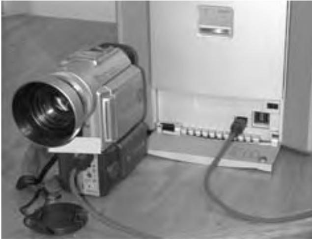
A camcorder connected to a computer's IEEE 1394 port.
