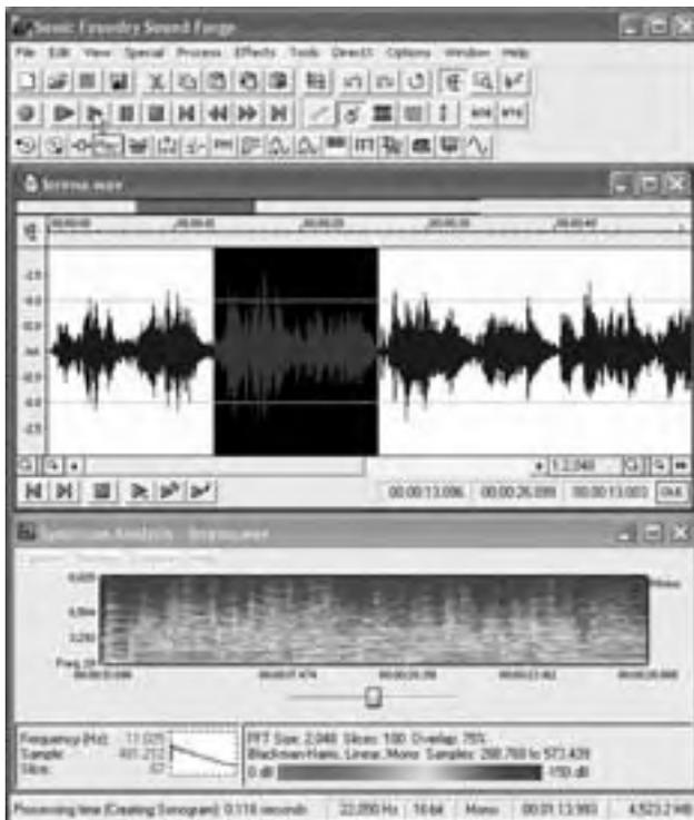
Here is a typical audio tool, Sound Forge from Sonic Foundry. This example shows a single-channel audio clip displayed as a waveform. A spectrum analysis is being performed on the clip to show the frequencies and overtones present in the recording.
