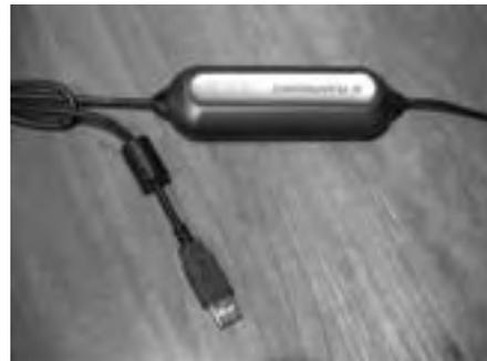
USB headphone/microphone combo and attached digitizing unit
