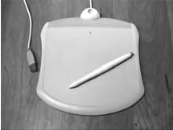
A stylus-tablet that connects to a computer's USB port.
